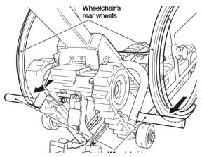
3. Move Wheelchair until Wheelchair's rear wheels lightly contact Wheelchair Support Tubes. Then set Wheelchair's parking brakes. 4. Move Wheelchair until Wheelchair's rear wheels lightly contact Wheelchair Support Tubes. Then set Wheelchair's parking brakes.
