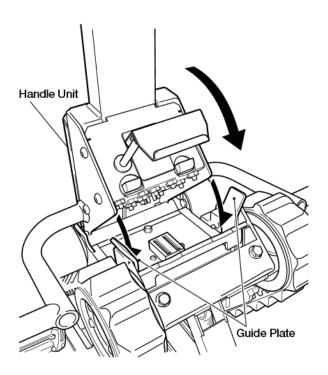
Check that Lock Unit functions correctly, and Handle Unit remains stowed when Handle is locked.
