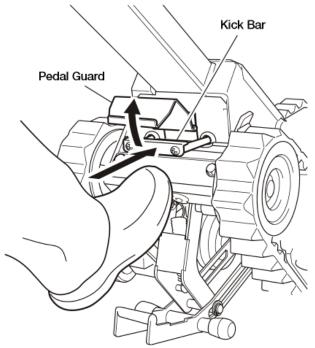
Check that there is no crack or other damage to Pedal Guard or Kick Bar and that they function normally.
