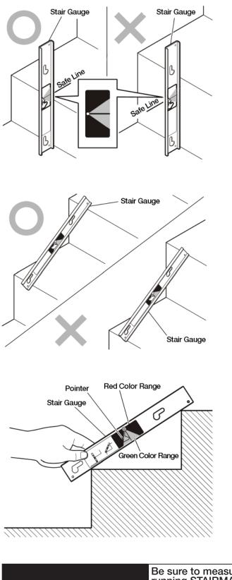
2. Put Stair Gauge vertically against the stair. Measure one stair's height. It is possible to use STAIRMATE if the height is less than Stair Gauge's Safe Line. Never use STAIRMATE on a stair if its height exceeds Stair Gauge's Safe Line.
