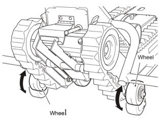
Check that there is no deformation or crack in Kick Stand and that it functions correctly.
