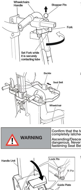
7. While pulling Stopper Pin, set Fork so that it secures Wheelchair's handle, and then the release Stopper Pin to lock Fork firmly.
