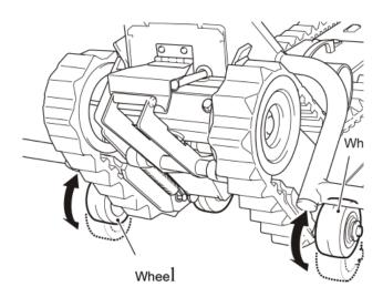
Check that there is no crack, wear or pitch error regarding Rubber Crawlers.
