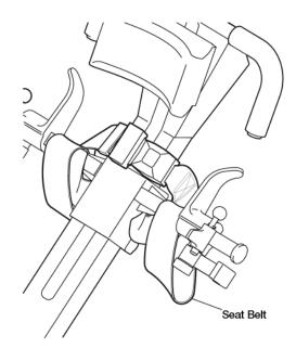
Check that there is no deformation or crack in any Seat Belt securing part and that Seat Belt is securely locked.
