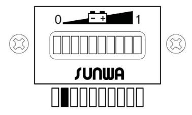
Check that the right end lamp of Battery Gauge is illuminated.
