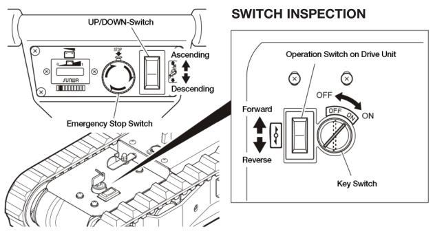
Check that all Switches function correctly.
